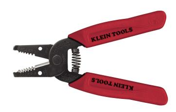
This Klein Tools Wire Stripper/Cutter cuts, strips, loops and gauges 16-26 AWG stranded wire. The precision-ground stripping holes cleanly cut wire and aid in easy removal of insulation. A narrow nose helps this tool fit easily into tight places.
