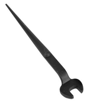
Forged from select alloy steel, the Klein Tools 7/8-Inch Nominal Opening Spud Wrench is designed to withstand high-leverage and heavy loads. It's designed for use with 1/2-Inch bolts and U.S. heavy nut types. The extra-duty head area gives maximum strength and durability. Plus, the continuous taper of the handle makes it easy to line up bolt holes.
