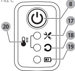
When the battery state of charge LED **19** is lit, regardless of color, the tool is ON.
