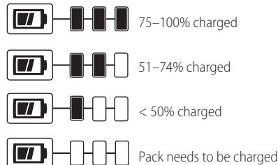
To activate the fuel gauge, press and hold the fuel gauge button. A combination of the three green LED lights will illuminate designating the level of charge left. When the level of charge in the battery is below the usable limit, the fuel gauge will not illuminate and the battery will need to be recharged.
