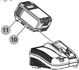
2. Insert the battery pack **10** into the charger, making sure the battery pack is fully seated in the charger. The red (charging) light will blink continuously indicating that the charging process has started.
